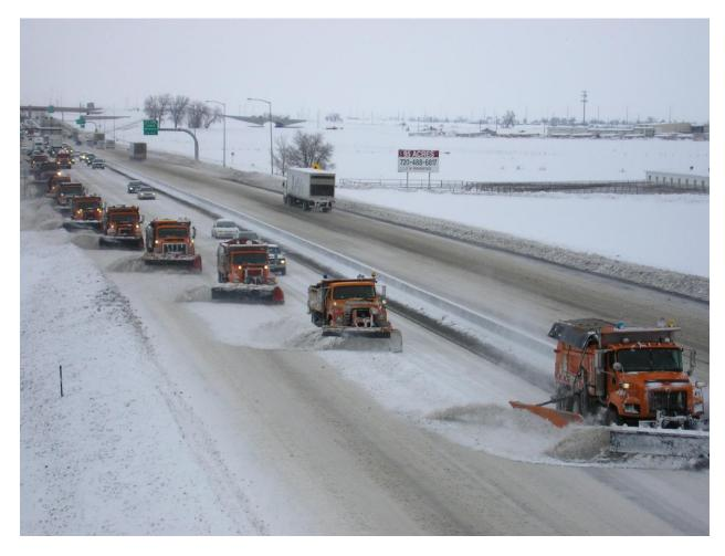
CDOT crews plow I-25 in tandem to pull snow away from areas such as walls and medians where drainage is poor. Snow and ice removal is a customer service CDOT offers that directly affects the traveling public.
