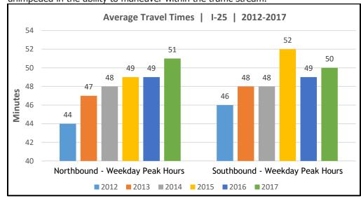
At left are average travel times per trip for Interstate 25 (between Northwest Parkway and C-470) from 2012-17. CDOT aims to limit the growth of travel times during peak weekday hours. The freeflow line is lower than chart measurements at 30 minutes.
