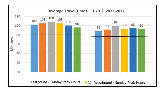
At left are the average travel times per trip for Interstate 70 (between Vail and C-470) from 2012-17. The black line indicates the free flow level for travel. The eastbound freeflow is 80 minutes and westbound is 78 minutes.
